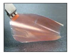
Nanodiamond-embedded devices could be used to deliver a broad range of therapeutics for the treatment of cancer and inflammation and for regenerative medicine. The extremely thin and flexible devices also can be customized to any shape and thickness.
