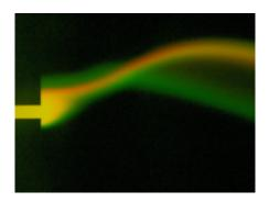
Left: the capillary electrophoresis chip developed by Zalewski. Right: separation of a mixture of rhodamine B and fluorescein. The substances are separated in two dimensions and come out in a wavelike movement.
