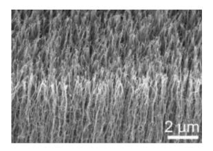
Typical side view of the inverted vertically-aligned multi-walled carbon nanotube film without top entangled segments before adhesion measurements. Image courtesy of Liangti Qu
