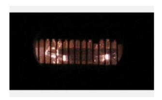
The silicon sample is shown in the resonator used in the experiment. The team created a system that used both the electron and nucleus of a phosphorous atom embedded in a silicon crystal. Both the electron and nucleus behaved as tiny quantum magnets capable of storing quantum information. This allows information to stay intact for over a second, an important threshold in the development of quantum computing. Courtesy of Stephen A. Lyon, Princeton University
