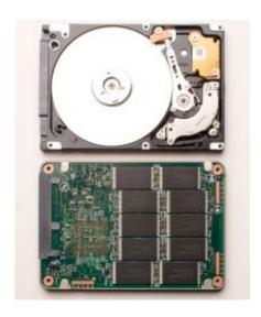
Comparison of the inside of a hard disk drive (HDD) versus a solid-state drive (SSD), which has no moving parts for quieter and more reliable operation.
