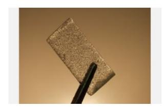
The bubbles visable in this piece from an Antarctic ice core sample contain carbon dioxide and other gases that were trapped in the ice when formed thousands of years ago. Researchers carefully crush the piece and capture the gases that escape when the bubbles break. This allows them to better understand what carbon dioxide levels were over time. Courtesy of Oregon State University
