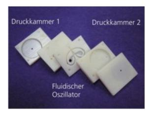
The resulting pressure fluctuation is then converted into electrical energy by piezoceramics in the pressure chambers. Credit: Fraunhofer TEG
