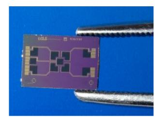
The LCLS total energy sensor will sit directly in the X-ray beam during commissioning to help calibrate diagnostic equipment. Photo by Brad Plummer
