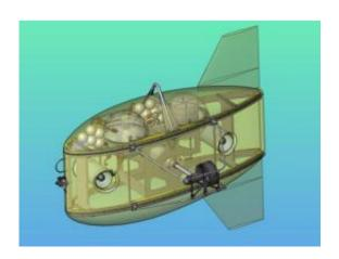
Schematic shows Odyssey IV, a small, inexpensive, MIT-designed robotic submarine that can hover in place like a helicopter. Image courtesy / MIT Sea Grant AUV Lab
