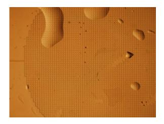
This optical micrograph of a synthetic tree shows a "trunk" channel entering from the left into a network of microchannels in the "leaf," or "root," network. The channels are approximately 100 micrometers wide, and total field of view is approximately 1.5 centimeters wide. Image: Tobias Wheeler
