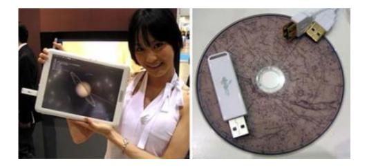
StellarWindow consists of a USB stick containing a compass and accelerometer that can identify which celestial objects a user is pointing their computer at. Credit: Hobby Media.
