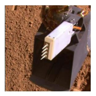
Phoenix inserted the four needles of its thermal and conductivity probe into Martian soil during the 98th Martian day, or sol, of the mission and left it in place until Sol 99 (Sept. 4, 2008). Image credit: NASA/JPL-Caltech/University of Arizona/Texas A&M University
