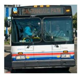
The driver controlled braking and speed, while magnets guided steering as this bus made a demonstration run along a San Leandro street. (Bill Stone/California PATH, UC Berkeley photo)
