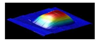
Scientists have developed the world's thinnest balloon that is impermeable to even the smallest gas molecules. Above is a multi-layer graphene membrane that could be used in various applications, including filters and sensors. Image: Jonathan Alden
