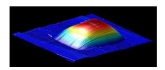
Scientists have developed the world's thinnest balloon that is impermeable to even the smallest gas molecules. Above is a multi-layer graphene membrane that could be used in various applications, including filters and sensors. Image: Jonathan Alden
