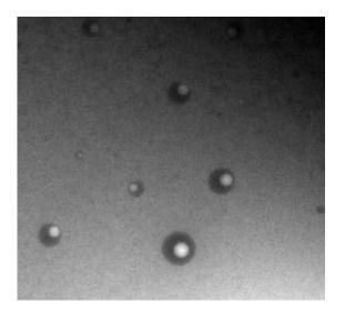
In this electron micrograph image, the white areas are water droplets; they are contained within darker oil droplets. The droplets are in water. (Credit: Jarrod Hanson/UCLA Bioengineering)
