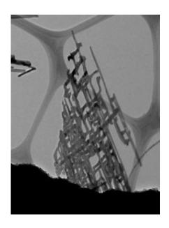
Researchers at Boston College report creating nanonets, pictured here magnified 50,000 times. The novel nano-scale structure was grown from titanium and silicon in a two-dimensional network of wires that resembles flat, rectangular netting. Credit: Angewandte Chemie International
