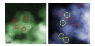
Electron micrographs showing inactive (left) and active (right) catalysts consisting of gold particles absorbed on iron oxide. The red circles indicate the presence of individual gold atoms. The yellow circles show the location of subnanometer gold clusters that can effectively catalyze the conversion of carbon monoxide to carbon dioxide. One nanometer is about half the size of a DNA molecule. (Color added for clarity) Credit: Lehigh University Center for Advanced Materials and Nanotechnology
