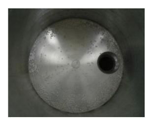
The researchers filled a cylindrical bucket with glass beads and measured the force required to lift the beads. Credit: Costantino, Penn State
