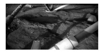
The Robotic Arm Camera on the Phoenix Mars Lander took this view under the spacecraft on Sept. 1, 2008, the 97th Martian day of the mission after landing. The lander leg strut at upper left features clumps larger than those seen three months ago. Also, exposed patches beneath the lander are darker than they used to be. (NASA/JPL-Calech/University of Arizona/Max Planck Institute)
