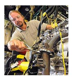
Argonne mechanical engineer Thomas Wallner adjusts Argonne's "omnivorous engine," an automobile engine that Wallner and his colleagues have tailored to efficiently run on blends of gasoline, ethanol and butanol.
