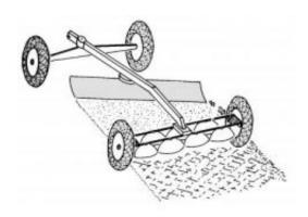
Lunar dust melts readily when exposed to microwave energy. Professor Larry Taylor of the University of Tennessee envisions a lunar paver fitted with microwave generators that could sinter, or melt, lunar soils into landing strips or roads. Credit: Larry Taylor
