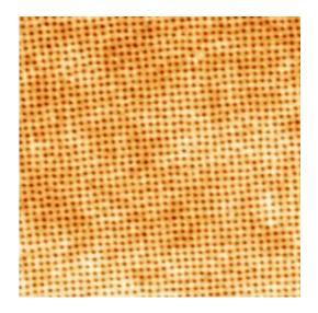
Atomic Force Microscope image of a square array of 15nm pores formed by the new technology.
