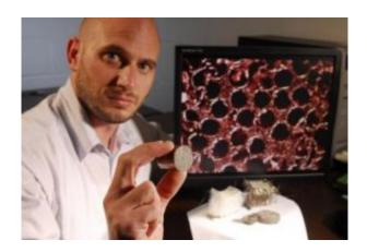
Georgia Tech Research Institute research engineer Jason Nadler has developed a new microchanneled material that reduces aircraft engine noise by wearing it down through a process called viscous shear. Georgia Tech Photo: Gary Meek
