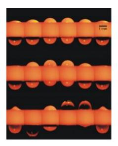
A new technique for creating liquid lenses with water and sound could enable a new generation of low cost, lightweight, energy efficient cameras. This series of time-lapse photos shows how the lens, made up of two droplets of water vibrating at a high speed, changes shape and, in turn, moves in and out of focus. The time between frames is four milliseconds. Image- Rensselaer/Carlos A. Lopez
