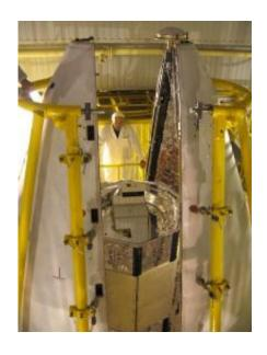
GOCE being encapsulated in the two half-shells of the launcher's fairing. Credit: ESA
