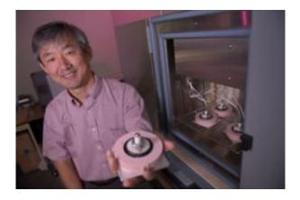
Sang-Soo Kim demonstrates the Asphalt Binder Cracking Device. Photo by: Rick Fatica
