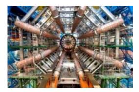
The Atlas experiment under construction at the LHC site, deep beneath the Alps. The large tubes that surround the empty space are magnets used to control the direction of subatomic particles. Credit: AFTAU
