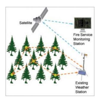
The sensor system produces enough electricity to allow the trees' temperature and humidity sensors to regularly and wirelessly transmit signals. Each signal hops from one sensor to another, until it reaches an existing weather station that beams the data by satellite to a forestry command center. Graphic / Rebecca Macri
