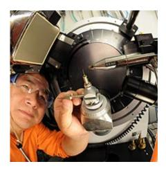
Scientist Yu-Sheng Chen calibrates the needle of the X-ray diffraction machine at ChemMatCARS in the Advanced Photon Source. The beamline is the only place in the U.S. able to examine the small crystals of compound that may be able to identify biological and chemical weapons.
