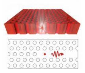
Photonic crystal membrane waveguide with an emitting quantum dot (red dot) in side-view (upper image) and top-view (lower image). An excited quantum dot emits one photon at a time, which is directed into the waveguide with very high efficiency. Image: Peter Lodahl
