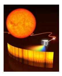
An optical fiber is used to guide the light collected in telescopes to the spectrograph, where it is split up into its individual colors. These are then compared with the frequency comb -- seen here as equally spaced lines -- to obtain an accurate determination of the color. Credit: ESO
