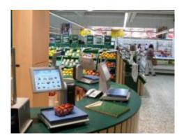
The intelligent self-service scales automatically recognize which type of fruit or vegetable has been placed on them. (c) Fraunhofer IITB
