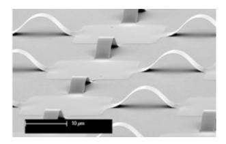
This image shows a close-up view of the silicon photodetector pixels and electronics interconnected by arc-shaped ribbons. The scale bar represents 10 micrometers (millionths of a meter). Credit: Northwestern University and University of Illinois
