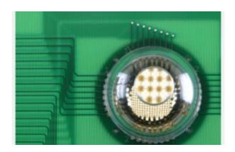
The electronic-eye camera developed by researchers from the University of Illinois at Urbana-Champaign and Northwestern University. The array of pixels is visible through the magnified image created by the lens. Image: Beckman Institute, University of Illinois
