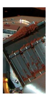
This false-color image shows a soil sample after being delivered to a gap between partially opened doors on the lander's Thermal and Evolved-Gas Analyzer. Image credit: NASA/JPL-Caltech/University of Arizona/Texas A&M University
