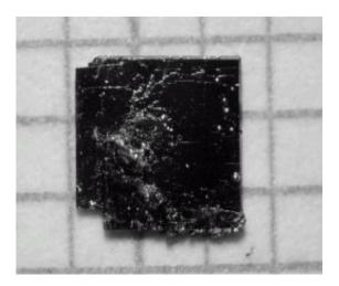
A sample of a potassium-doped iron arsenide superconductor, shown on a millimeter grid. Image courtesy the American Physical Society [N. Ni et al. (10 July 2008). Anisotropic thermodynamic and transport properties of single-crystalline Ba1?xKxFe2As2 (x=0 and 0.45). Physical Review B, Vol 78, p014507, Fig 1]
