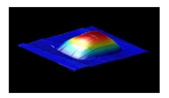
Scientists have developed the world's thinnest balloon that is impermeable to even the smallest gas molecules. Above is a multi-layer graphene membrane that could be used in various applications, including filters and sensors. Image: Jonathan Alden
