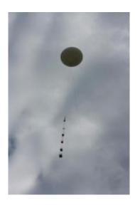
The high-altitude balloon carrying a radiation detector, high-resolution camera, sensors for temperature, pressure and humidity, and a GPS launches from OSU in Stillwater. Image: Dr. Jamey Jacob
