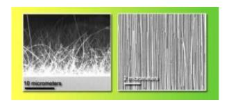
Randomly oriented nanowires, on the growth substrate at left, are having a "bad hair day." But after contact printing, the nanowires on the receiver substrate are highly aligned. (Javey group) Credit: Lawrence Berkeley National Laboratory; University of California at Berkeley
