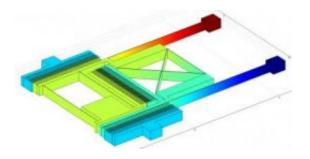
This illustration depicts a tiny device called a monolithic comb drive, which might be used as a high-precision "nanopositioner" for such uses as biological sensors, computer hard drives and other possible applications. The device was created by Jason Vaughn Clark, an assistant professor of electrical and computer engineering and mechanical engineering at Purdue University. Credit: Birck Nanotechnology Center, Purdue University
