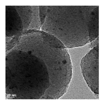
In this transmission electron micrograph of the mesoporous nanospheres, the nano-scale catalyst particles show up as the dark spots. Using particles this small (~ 3nm) increases the overall surface area of the catalyst by roughly 100 times.
