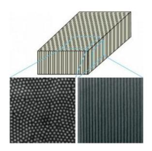
Shown is a schematic and two scanning electron microscope images with top and side views of a metamaterial developed by UC Berkeley researchers. The material is composed of parallel nanowires embedded inside porous aluminum oxide. As visible light passes through the material, it is bent backwards in a phenomenon known as negative refraction. Credit: Image by Jie Yao, UC Berkeley
