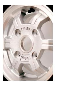
An alloy wheel produced using the T-Mag die casting technology, one of the CSIRO technologies for producing light-weight car parts. Image: CSIRO
