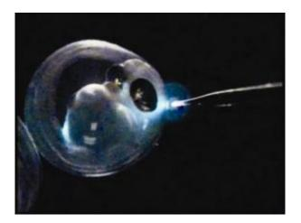
Purdue University researchers use an optical electrode, or optrode, right, to measure oxygen consumption in a two-day-old fathead minnow embryo, about half the width of the head of a pin. By watching for worrisome changes within these tiny fish eggs, the technology could be used as a monitoring tool against environmental contamination or even biological weapons. Image: Marshall Porterfield
