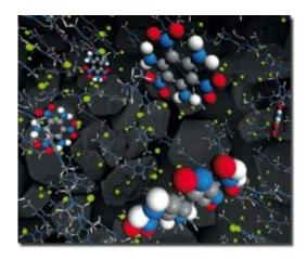
Fluoride ionic liquid as a novel super-efficient solvent can lead to high-quality single crystals of technologically important materials. The molecules in red, white, blue and gray are the explosive, TATB. The green balls (fluoride anions) and the gray and blue sticks (cations), act as the solvent. The rocks in the background are TATB crystals.
