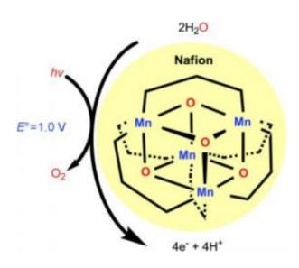
A manganese-oxo complex with a cubic {Mn4O4}7+ core catalyzes the electrooxidation of water when suspended within the aqueous channels of a Nafion membrane (see picture). Illumination with visible light under an applied potential of 1.0 V (vs Ag/AgCl) generates current over one thousand turnovers. The catalytically active species arises from photolysis and subsequent dissociation of the manganese complex. (c) Wiley-VCH 2008
