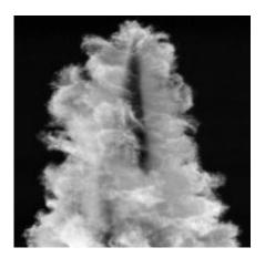
A scanning electron microscope image of a metal electrode (dark region in center of image) coated with carbon nanotubes.
