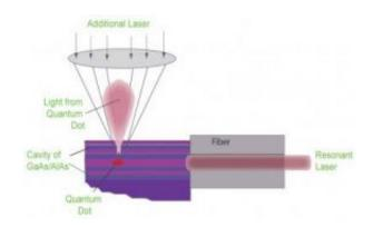
Schematic of NIST-JQI experimental set up. Orienting the resonant laser at a right angle to the quantum dot light minimizes scattering. Image: Solomon/NIST
