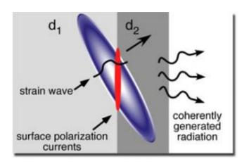
Electromagnetic radiation is produced when an acoustic wave (purple) generates electric currents (red) as it propagates past an interface between two piezoelectric materials. The radiation propagates outside of the materials and can be detected to determine the shape of the acoustic wave with nearly atomic scale resolution.
