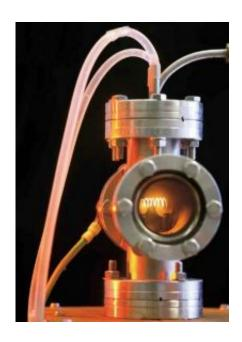
A small twisted wire, just like the filament in an incandescent bulb, but made of silver, forms the basis for the special silver particles. Credit: Sam Rentmeester/FMAX
