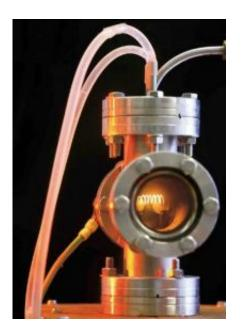
A small twisted wire, just like the filament in an incandescent bulb, but made of silver, forms the basis for the special silver particles. Credit: Sam Rentmeester/FMAX
