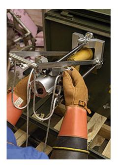
Johns Hopkins undergraduates designed this tool to allow electric utility workers to disconnect a power line from a residential transformer box with reduced risk of injury. Photo by Will Kirk
